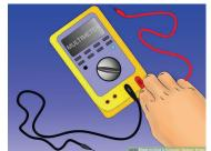
**Testing for a Slow Drain on the Battery**: Perhaps everything checks well but the battery keeps running down when you leave the boat for a few days or weeks. You might have something that is slowly drawing current. This could be a radio, clock, or some other device that is not
